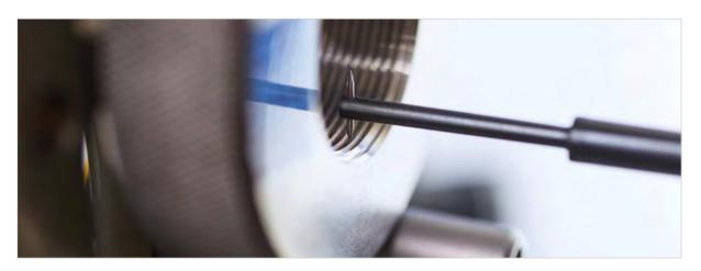
Older quality control methods on the production line, e.g. physical thread gauges, are being replaced more and more by actual measurement methods. Parameters whose evaluability was limited when using such gauges can now be quickly and easily documented.
