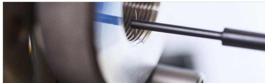
in the thread root and the roughness of the thread flanks, is only possible by modern, scanning data acquisition. Parameters that cannot be measured by „gauging“ can be determined quickly and reliably, recorded, and monitored in compliance with tolerances. Optical measurement is only possible to a limited extent due to the overlap caused by the thread pitch.
