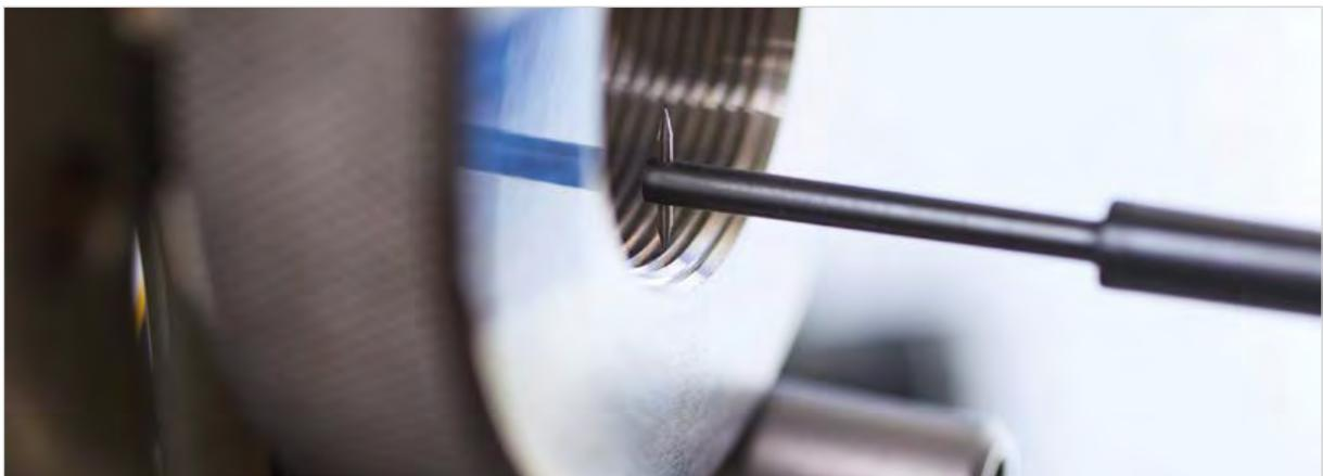
Older quality control methods on the production line, e.g. physical thread gauges, are being replaced more and more by actual measurement methods. Parameters whose evaluability was limited when using such gauges can now be quickly and easily documented.
